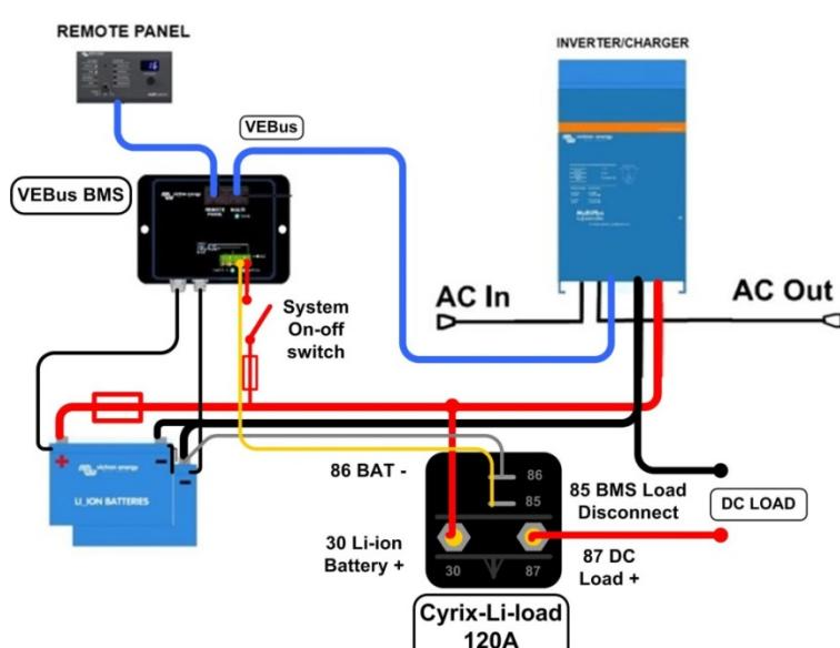
Figure 5: System with MultiPlus and DC loads
