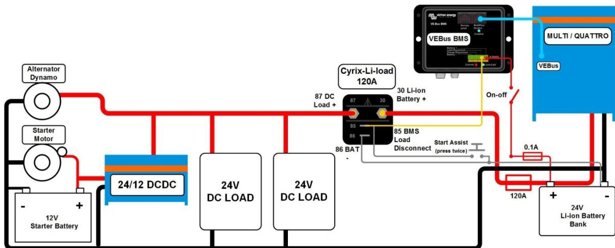
Figure 9: System example for a boat or vehicle with a 24 V Li-ion system, a 24 V alternator and a 12V starter battery.
