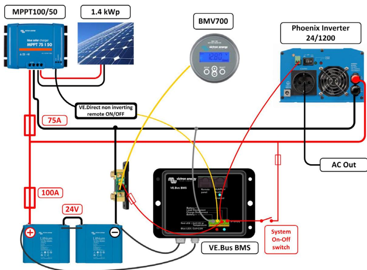
Figure 10: Solar application with an MPPT with VE.Direct port and a Phoenix Inverter 24/1200.
