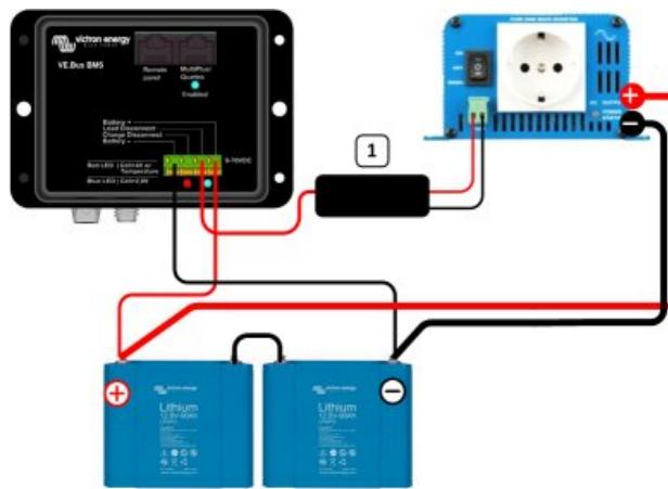
**Loads for which a Inverting remote on-off cable is needed**
