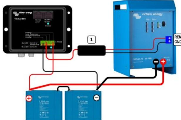
**For Skylla TG battery chargers a Non inverting remote on-off cable Is needed**
