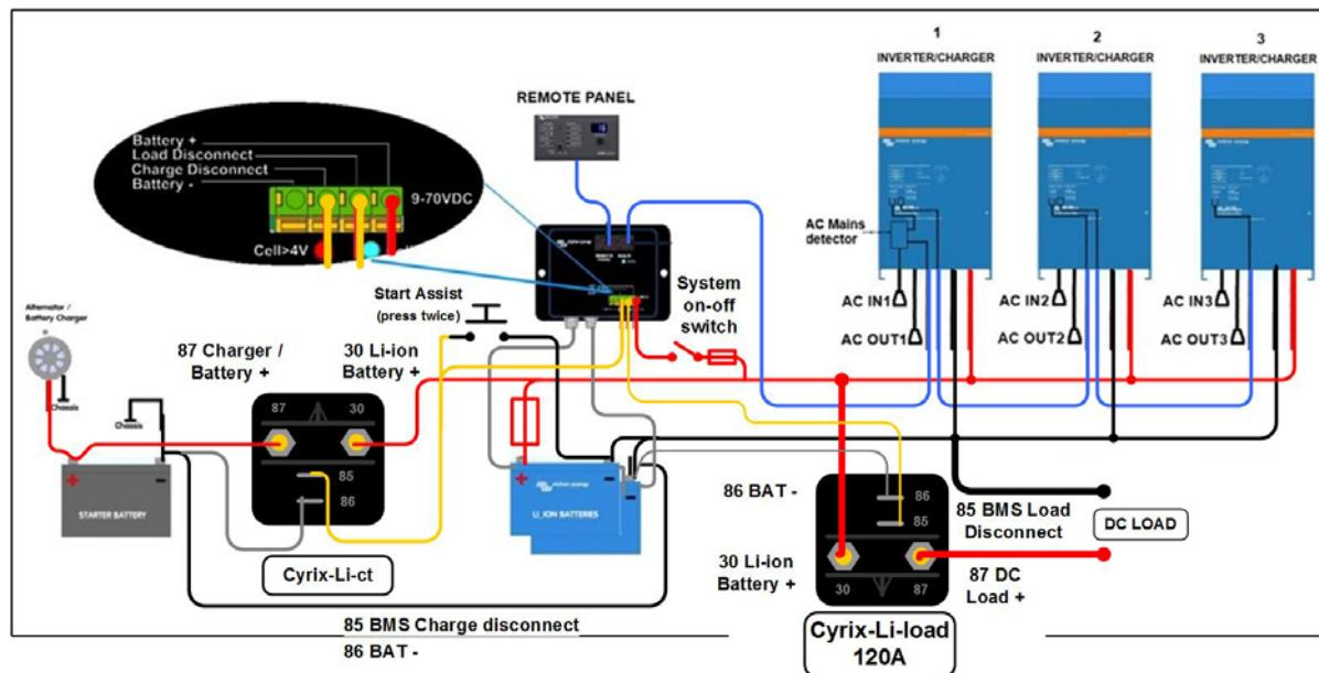
Figure 8: System example for a boat or vehicle with a three phase inverter/charger configuration (DC fuses not shown, except for the the Li-ion battery fuse)
