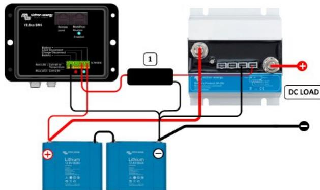
**Load disconnect switch for which a Non inverting remote on-off cable is needed**
