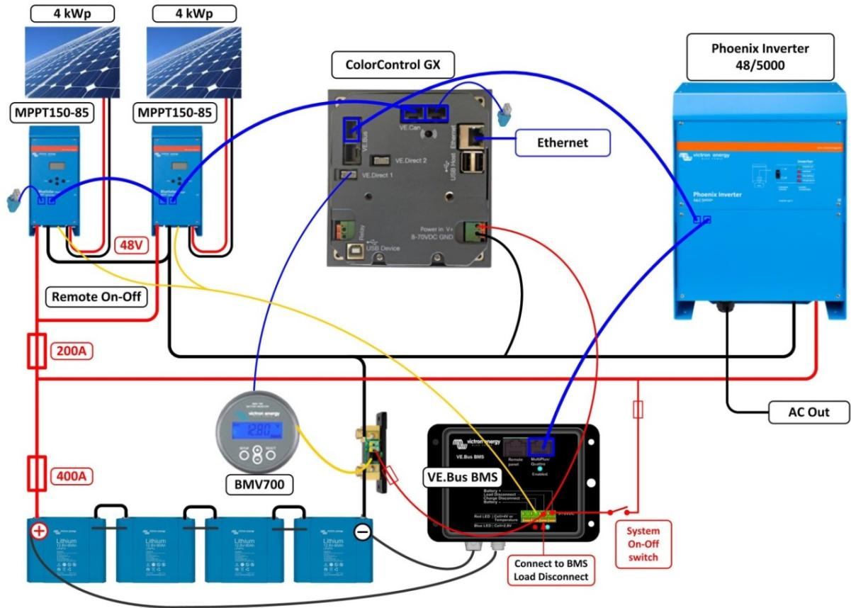
Figure 11: Solar application with two MPPT 150/85
